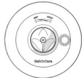
10. Fit the handle and fasten so the arrow shape on top of the handle matches the marking on the faceplate.
