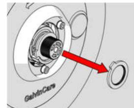
3. Remove the upper brass ring. Make sure the control rod doesn't rotate during the next steps.
