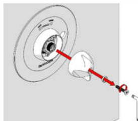
2. Unscrew the tamper proof screw from handle. Pull out handle assembly from the body
