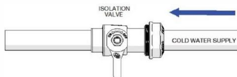
Restore the cold-water supply to the valve. After the mixed water temperature has stabilised note the outlet temperature ensuring the outlet temperature has re-established. The time taken to stabilise the temperature should not exceed the maximum time set out in the applicable standard or code of practice for each state.
