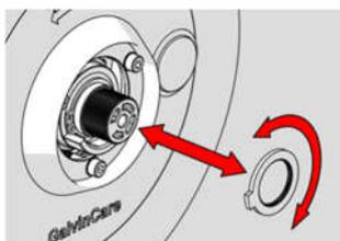
4. Remove the lower brass ring (temperature setting ring) and rotate the brass ring clockwise to increase temperature or anti-clockwise to decrease. Refit to spline in new position.
