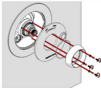
1. To isolate the shower, remove the handle and flange by unscrewing and carefully remove the inner faceplate and o-ring. (As shown)
