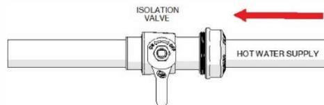
The outlet flow should quickly reduce to be less than 0.4L/min following the isolation. The volume of mixed water discharged for a period of between 5-35 seconds should be measured and should not exceed the maximum volume set out in the applicable standard or code of practice for each state.
